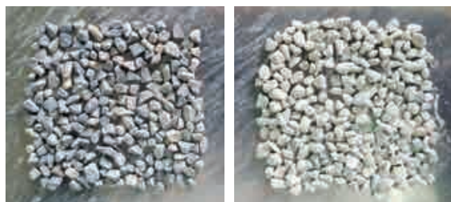
(Top) M-sand is more angular in shape compared to natural sand and quarry dust; (bottom left) washed M-sand; (bottom right) unwashed M-sand
